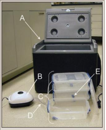
Fig. 1. Field maintenance and transport setup for cold-water amphibians. A) Thermoelectric cooler; B) air pump; C) latch containers; D) plastic tubing; and E) air stone. The thermoelectric cooler and air pump can be powered with conventional outlets when available. Alternatively, they can be plugged into a portable power system attached to a marine battery, providing cold temperatures and aeration over extended time periods.
